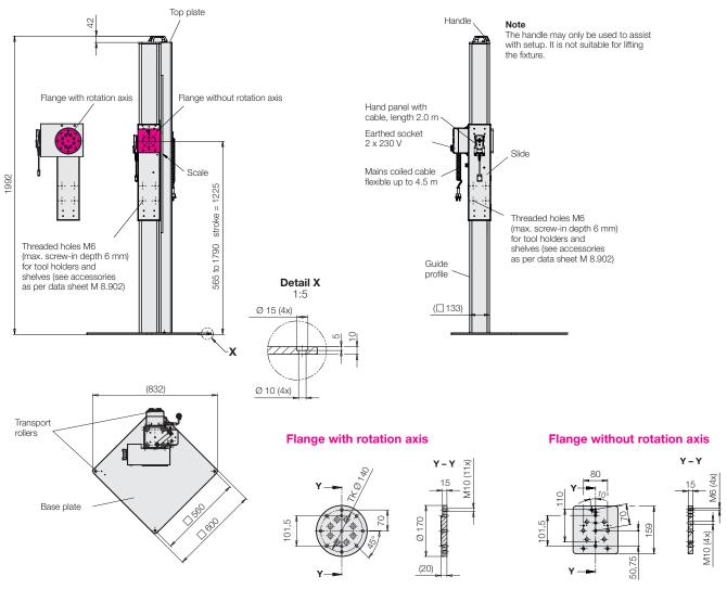
With internal threads for screwing on the universal fixture for clamping claws and 3-point
