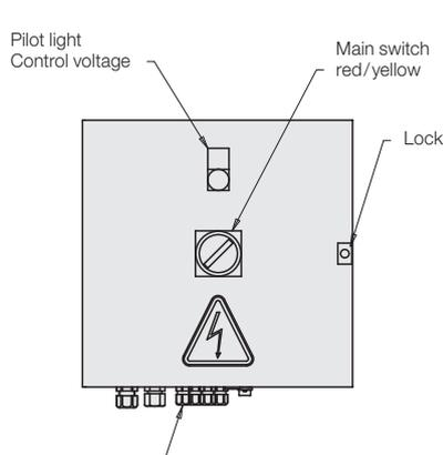
Tilting and control module are supplied with a 3 m long hard-wired cable.
